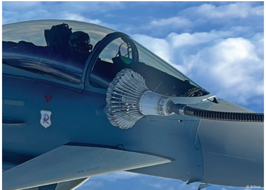
A Eurofighter is refuelled in flight by an A330 MRTT aircraft on 6 February 2023.
